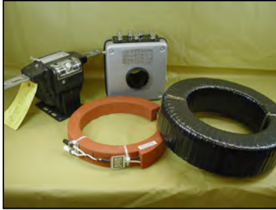
Lab Current Transformer.
